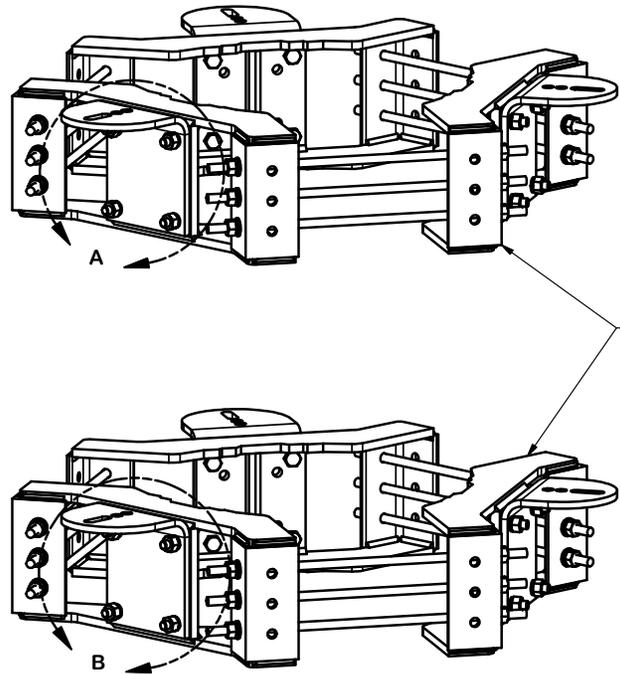
WILL WORK WITH ANY RING MOUNT WITH 5/8" BOLTS ON A 6" X 6" BOLT PATTERN
